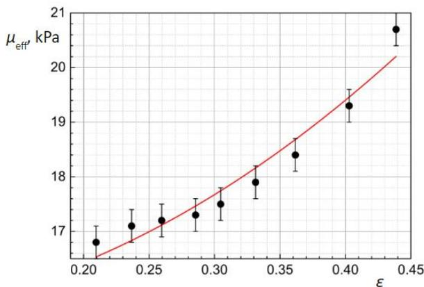
Figure 4. Measured effective shear modulus on the relative deformation
