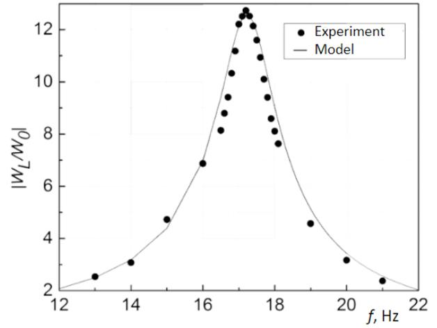
**Figure 6.** The frequency dependence of the ratio near the first resonance for the resonator without static load excited with the oscillations of amplitude  $W_0 = 1 \text{ m/s}^2$
