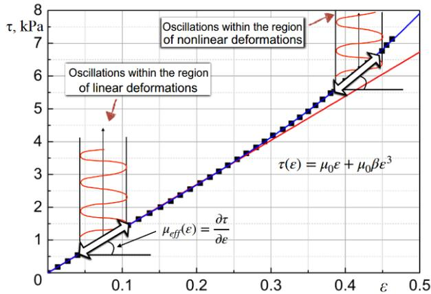
**Figure 8.** Measured shear stress  $\tau$  on the relative deformation  $\varepsilon$  (dots) approximated by the cubic parabola (blue line) and with the straight red line
