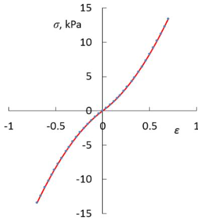
Figure 3. Measured shear stress on the relative deformation
