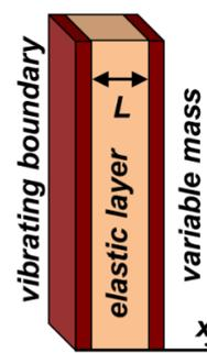
Figure 1. Gel-like resonator between two solid-state boundaries (elastic layer)
