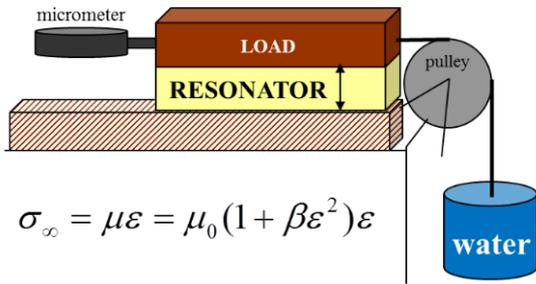
Figure 2. The experimental setup for static measurements of the shear stress on the relative deformation
