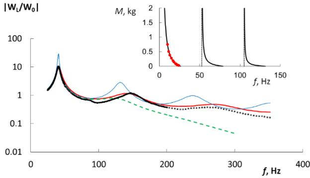
**Figure 5.** The ratio of the acceleration amplitudes  $|W_L/W_0|$  for the value  $W_0 = 1 \text{ m/s}^2$
