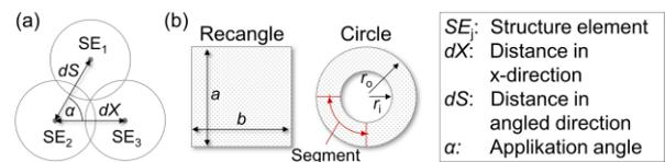
Figure 2. Geometrical arrangement of structure elements and replication in the NC-Code-Generator - according to [Meijer et al. 2021a]
