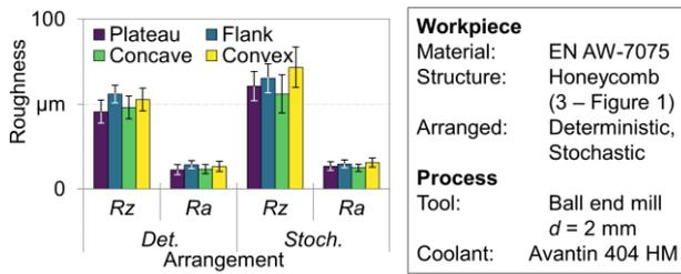
**Figure 9.** Structured demonstrator – Profile roughness parameters.
