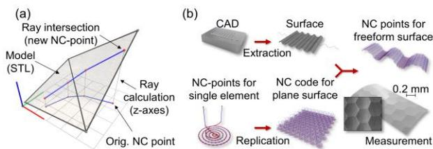
**Figure 3.** (a) NC-to-STL projection and (b) schematic process chain for structuring free-form surfaces - according to [Meijer et al. 2021a]
