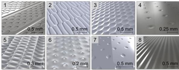
Figure 1. Selection of bionic motivated deterministic surface structures – according to [Meijer et al. 2021a]
