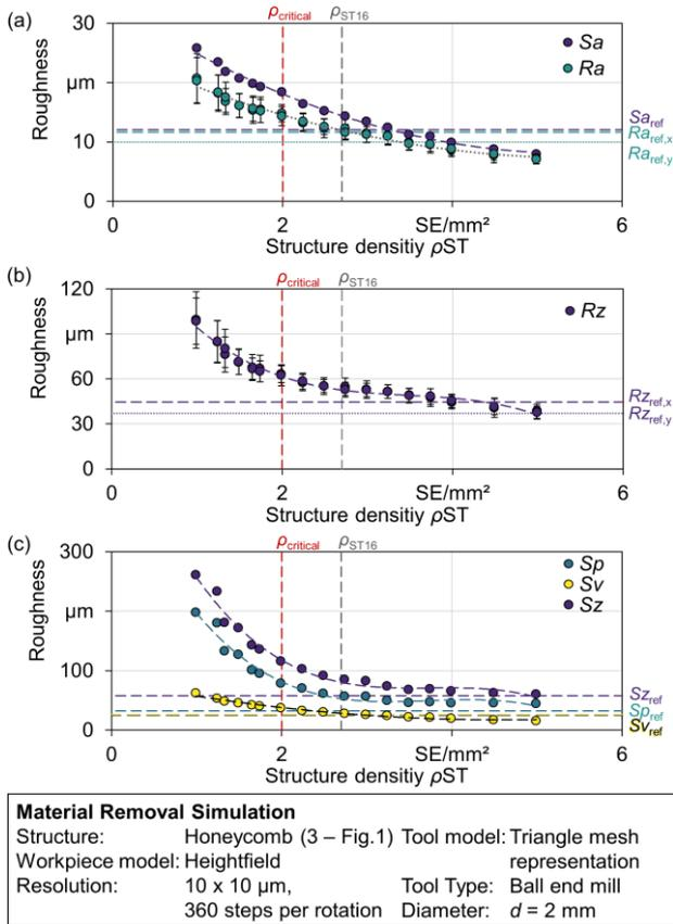
**Figure 6.** Influence of the structure density on the surface roughness: (a) arithmetic mean roughness  $Ra$  and arithmetic mean height  $Sa$ ; (b) maximum profile height  $Rz$ ; (c) maximum height  $Sz$ , maximum peak height  $Sp$ , and maximum pit height  $Sv$
