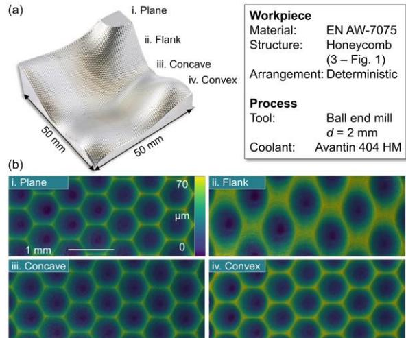
**Figure 7.** Structured demonstrator - arrangement of the bionically inspired structural variant according to a deterministic approach, which leads to a distortion of NC trajectories in critical areas such as the flank, and thus in reduced shape accuracy.
