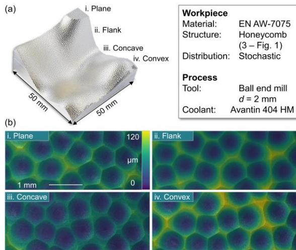
**Figure 8.** Structured demonstrator - arrangement of the bionically inspired structural variant according to a stochastic approach that leads to a quasi-homogeneous roughness even in critical areas such as steep flanks by allowing slight shape inaccuracies of the structure elements.
