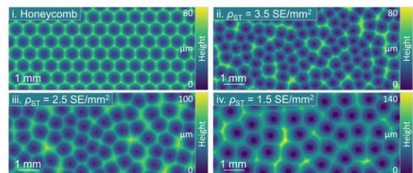
Figure 5. Topographies of stochastic structures with varying structure density compared to the deterministic honeycomb surface structure
