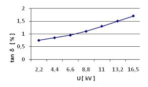
Figure 5. Process tan  $\delta$  loss factor – insulation Calmica 70 0867; t = 2,3 mm
