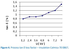
Figure 4. Process tan  $\delta$  loss factor – insulation Calmica 70 0867; t = 1,6 mm
