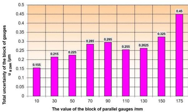
Figure 7. Total uncertainties of the block of parallel gauges.
