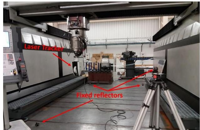
Fig. 3 Integrated Multilateration on a Zayer Memphis MT.
