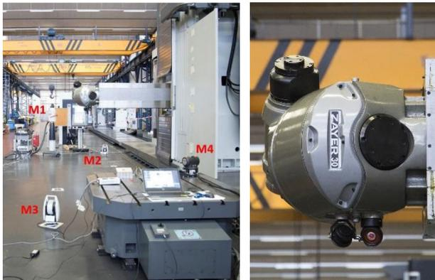
Fig. 2 Simultaneous Multilateration on a ZAYER KAIROS MT.
