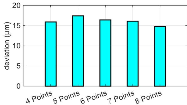
Fig. 5 Influence of the number of fiducial points on the MIIM expanded measurement uncertainty.
