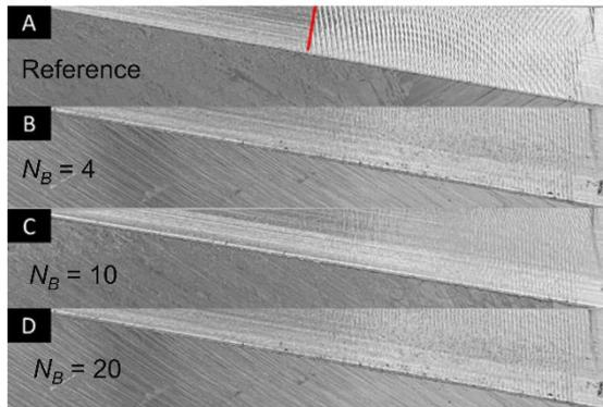
Fig. 20: Stability limit of Reference tool, and tool variants with different number of structure elements.
