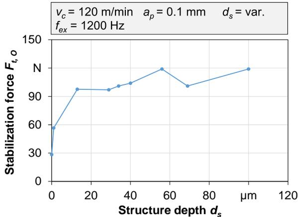
Fig. 11: Measured dynamic part of tangential force.
