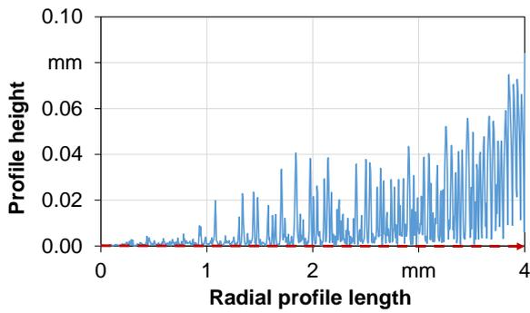
Fig. 16: Profile height along the main oscillation vector for  $d_s = 100 \mu\text{m}$ ,  $f_z = 0.12 \text{ mm}$ .
