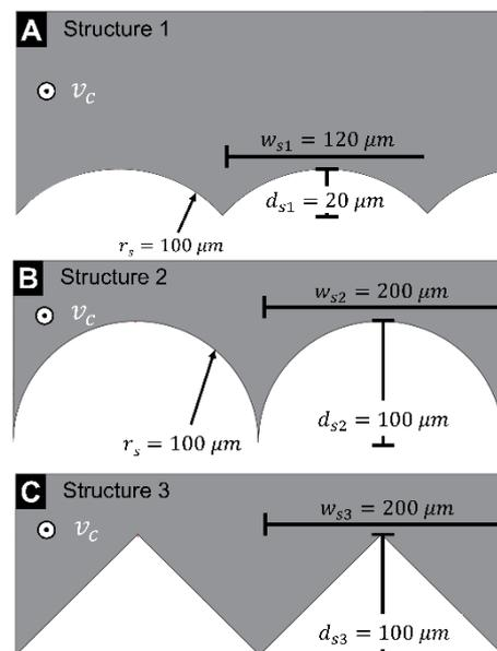
Fig. 3: Geometry of the observed structure variants.
