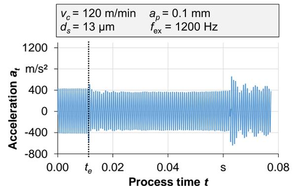
Fig. 10: Acceleration in direction of dynamic excitation.
