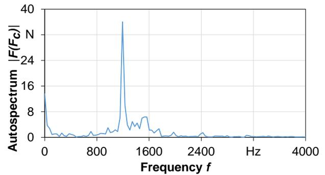
Fig. 9: Autospectrum of the cutting force component  $F_c$ .
