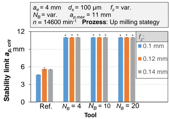
Fig. 21: Stability limit depending on the tool and the feed per tooth.
