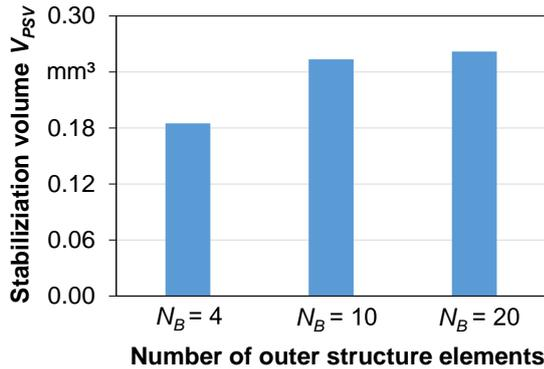
Fig. 17: Potential stabilization volume depending on the number of outer structure elements.
