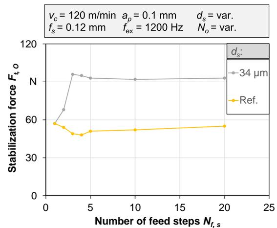
Fig. 13: Measured dynamic part of the tangential force with respect to number of feed steps.
