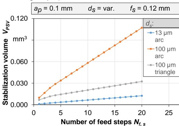
Fig. 5 Potential stabilization volume in dependency of the number of feed steps.
