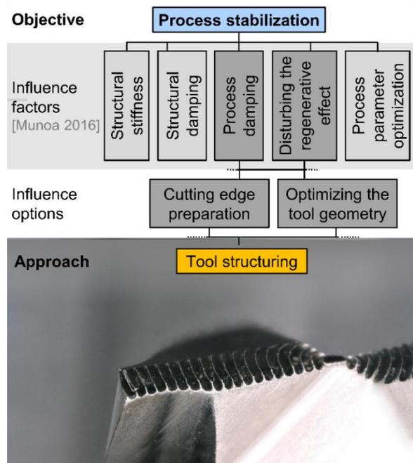
Fig. 1: Potential process stabilization approaches [Baumann 19].
