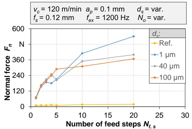
Fig. 12: Measured normal force  $F_n$  with respect to number of feed steps.
