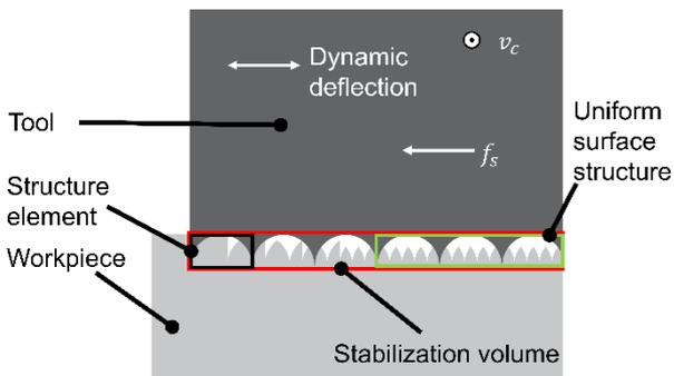
Fig. 4 Geometry of the Tool-workpiece interaction.
