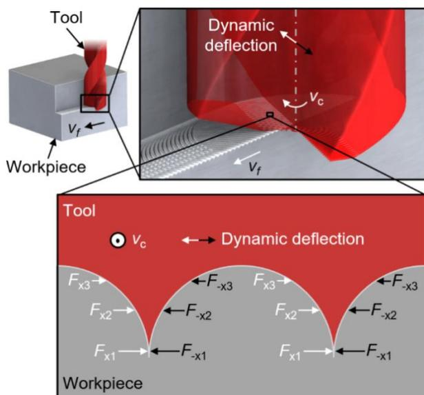
Fig. 2: Illustration of the working hypothesis [Baumann 19].
