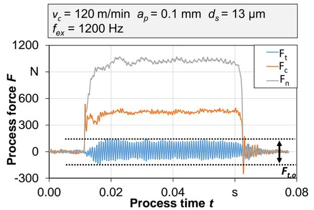
Fig. 8: Force progression during one cut of the analogy tests.
