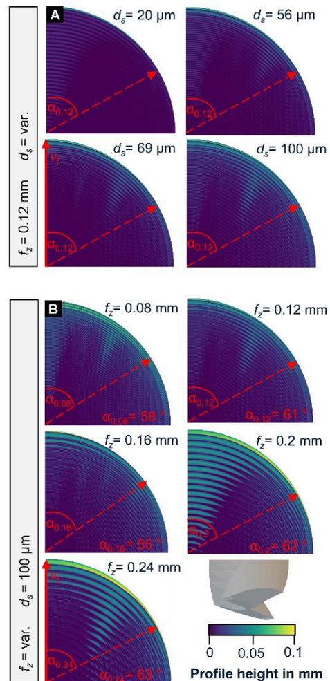
Fig. 15: Surface structure in dependence of (A) structure depth  $d_s$  and (B) feed per tooth  $f_z$  configuration.
