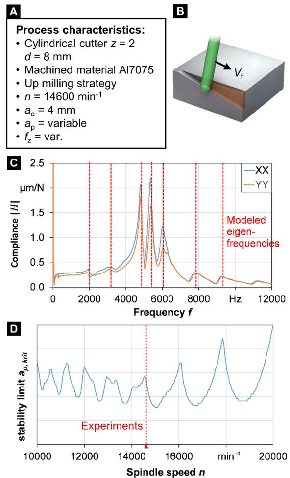
Fig. 19: Process design and parameter value selection based on simulations.
