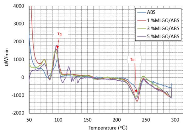
Figure 6. DSC thermogram for MLGO/ABS filament and print sample
