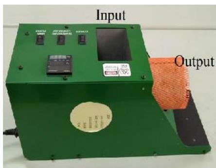
Figure 4. Single filament extruder
