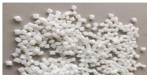
Figure 1. ABS plastic pellets
