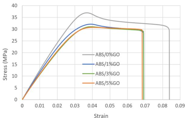
Figure 8. Stress and strain curves of printed samples printed from MLGO reinforced ABS plastic composite.
