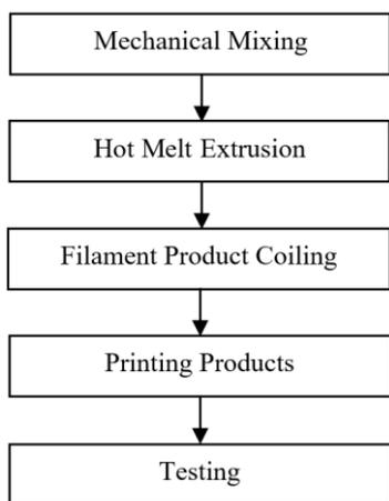
Figure 3. Filament fabrication and testing process
