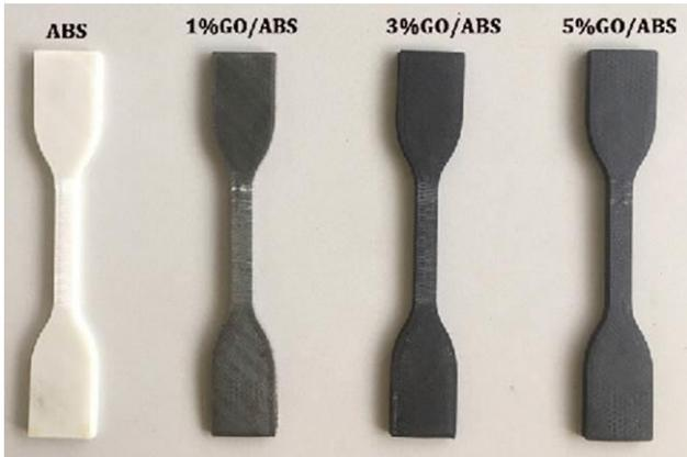
Figure 7. Tensile samples printed from MLGO reinforced ABS filament
