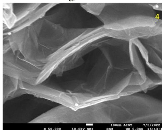
Figure 2. Multilayer graphite oxide
