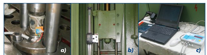
Figure 3. Experimental measuring system components – a) force transducer, b) displacement transducer Mitutoyo SD-60, c) frequency measuring amplifier IPRE2/VZV3
