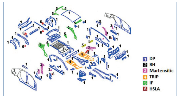
Figure 1. Use of various kinds of steel in the car's body [Parilak,2005] [worldautosteel.org]
