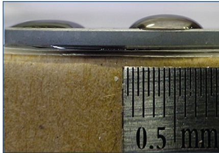
Figure 9. Measurement of wetting angle on piston ring
