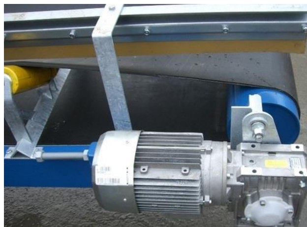
Figure 1. The use of asynchronous motors in belt conveyor [Svoboda 2015]
