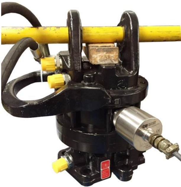
Figure 3. GV6 rotator with Model 731A accelerometer
