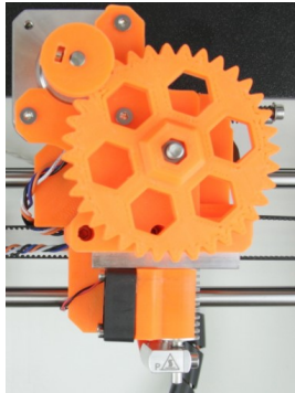
Figure 2. Example of the geared extruder [Prusa 2015]
