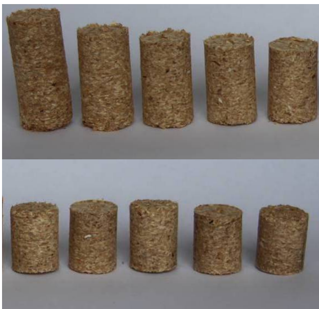
Figure 8. Briquettes from cherry tree sawdust produced with different acting pressures ( w_t=8\% ; L=2 mm). /Used pressures description - upper figure from left to right side: 31, 63, 95, 127 and 15 MPa; lower figure from left to right side: 191, 222, 254, 286, 318 MPa/
