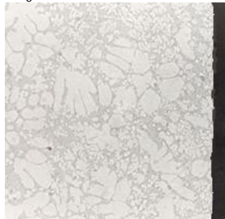
Figure 3. Macrostructure of sample edge (gravity casting) /250x/
