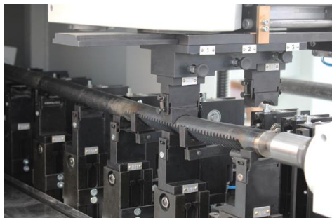
Figure 5. Alternative straightening machine [Galbadini 2012]
