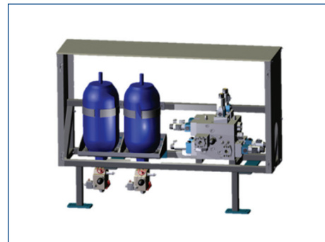
Figure 11. Some hydraulic parts of hydraulic recovery equipment
