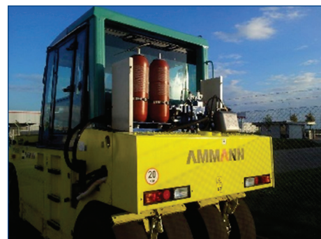
Figure 12. Road roller Ammann AP 240H equipped with hydraulic recovery module
