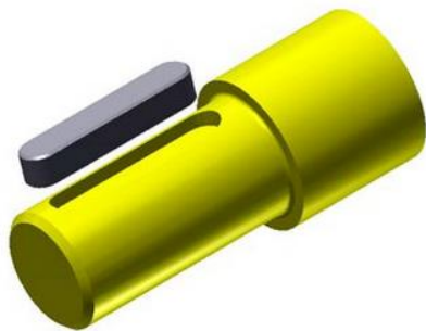
Figure 5. Model of the shaft connection with the hub by a tight spline
