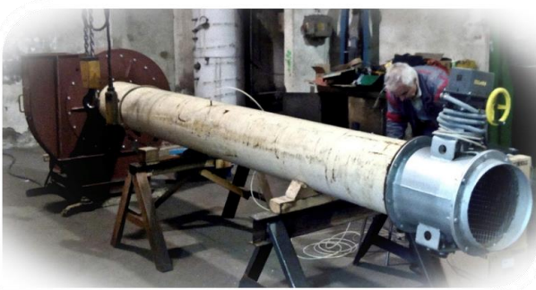
Figure 9 Measuring track for experimental tests on fans [Wittner 2015]
