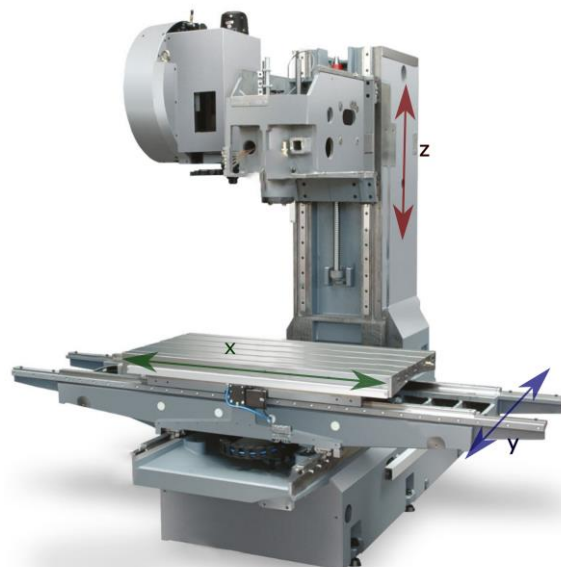
Figure 2. Working space of vertical machining center MCV 754QUICK
