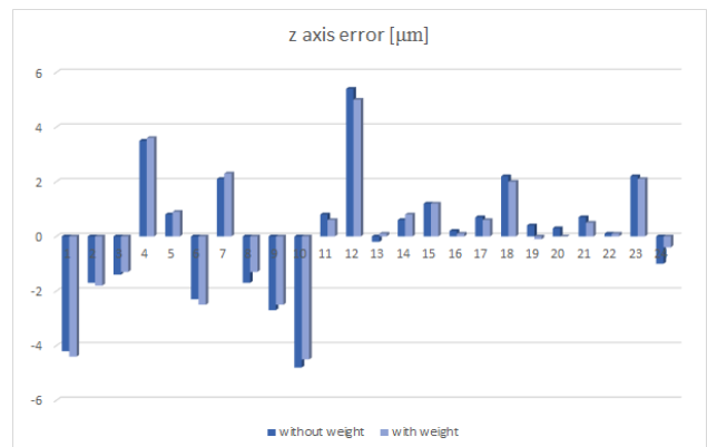
Figure 6. z axis errors [μm] for point 1-24 in work space
