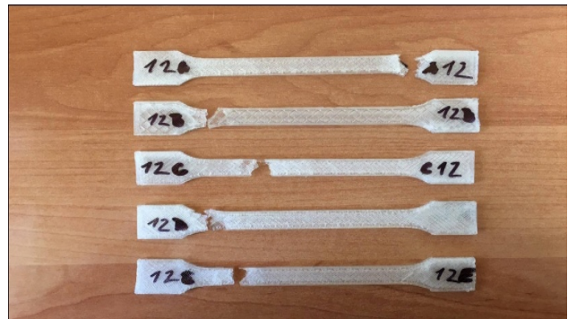
Figure 3. Test samples of clear PLA plastic horizontal in width after the test
