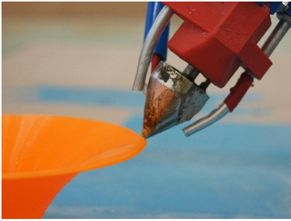
Figure 1. Tilting the print head in direction of the tangent surface
