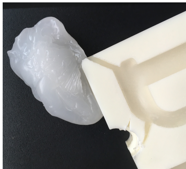
Figure 3. Damage of ABS insert during injection moulding
