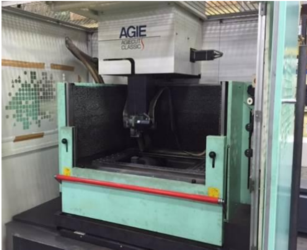
Figure 1. Electrical discharge machine Agiecut Classic 3S of the Swiss company GF Agie Charmilles used in the experiment
