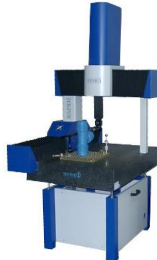
Figure 3. Thome Rapid CNC contact measuring device used in the experiment
