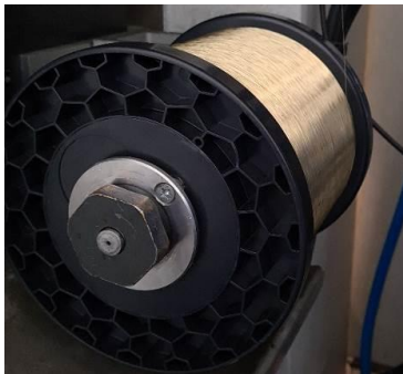
Figure 4. Wire tool electrode BEDRA MEGACUT type for TWO used in the experiment
