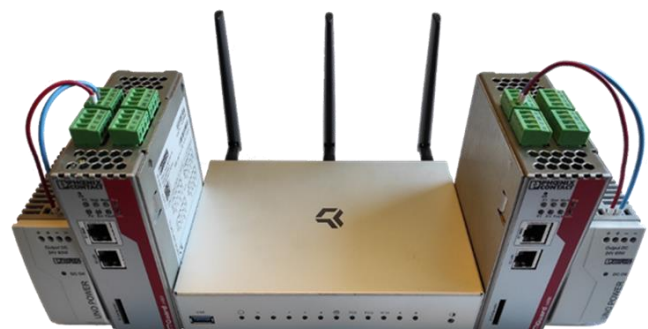
FIGURE 4. NETWORKING ELEMENTS USED IN THE STUDY (IN THE MIDDLE TURRIS OMNIA 2020, ALONG EDGES 2 X MQUARD RS4000)
