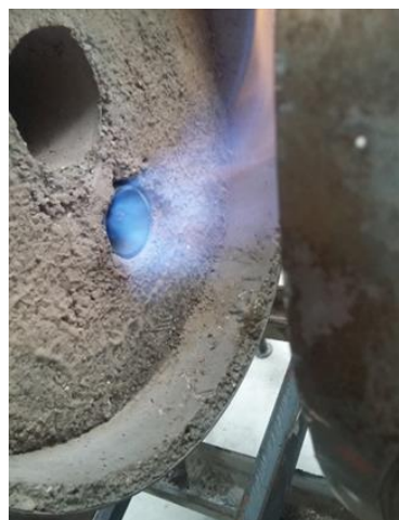
Figure 1. Physical model of a melting furnace with co-current supply of fuel and combustion air to the burner.
