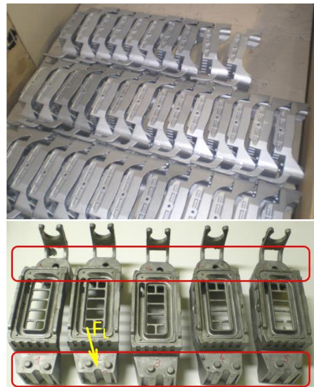
Figure 2. A group of realized castings with a marked sampling point for analyses and the direction of the load force F_1
