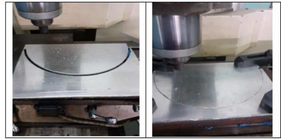
Figure 3. 6061 aluminum setting on lathe table ready for Friction Stir Welding radius joints
