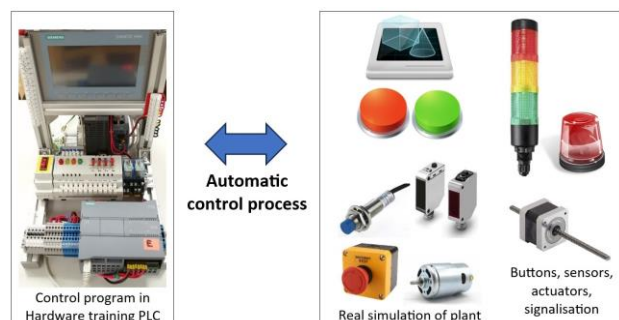
Figure 5. Hardware to User Activated Sensors model - Hardware PLC controls replacement hardware manually imitating the controlled system
