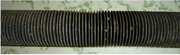
Figure 3. Cooler pipe with the ribs
