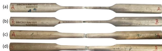
Figure 7. Fractured tensile specimens of (a) sample A and (b) sample B in the as-welded condition. Images (c) and (d) show corresponding specimens of aged welds.
