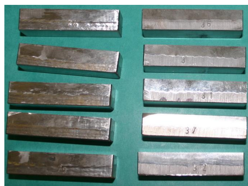
Figure 3. View of the cooked layers of the test samples
