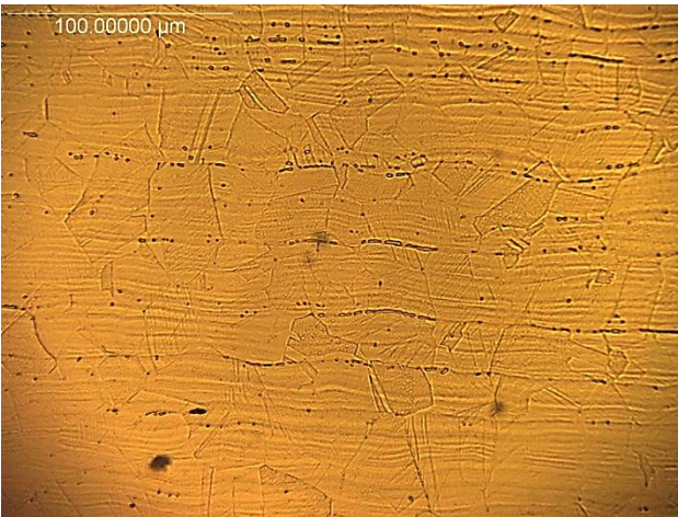
Figure 7. Photograph of the microstructure of the base material containing polyhedral grains of austenite with a small amount of delta ferrite (Microhardness: 200HV0.5)
