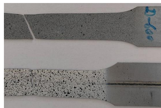
Figure 2c. Specimens after fracture – base material (top) and laser weld (bottom)
