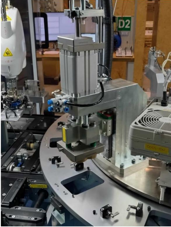
Figure 16. Seal test station [Belacek 2014]
