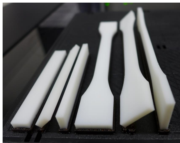
Figure 2. The bending (first three from left) and tensile specimens orientation relative to building platen (0°, 45°, 90°)
