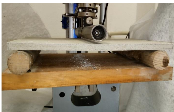
Figure 6. Positioning of test sample
