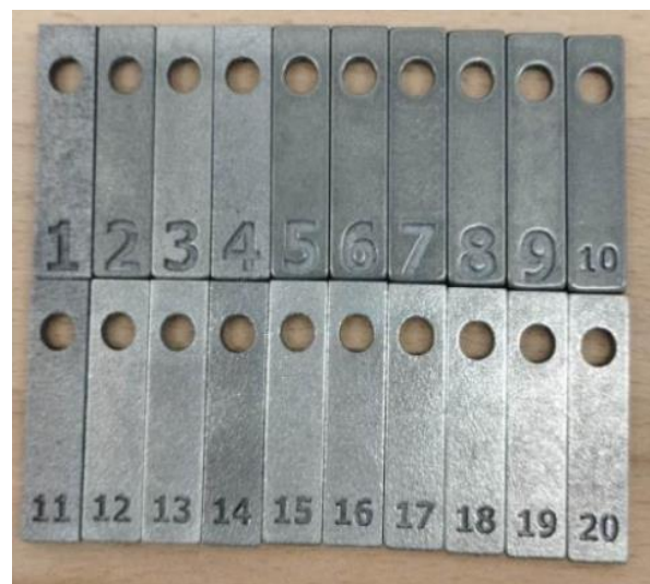
Fig. 4: AlSi10Mg samples material after printing
