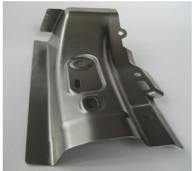
Fig. 1: Irregularly shaped stamping chosen for the evaluation of blank material influence on stamping springback
