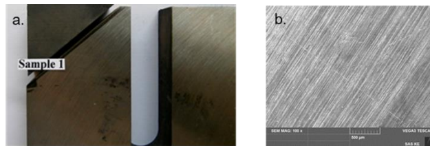
Fig. 4: Macroscopy of the ground surface of the knife sample (a.); tool surface grinding marks (SEM) (b.)
