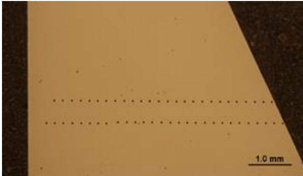
Fig. 3: Measurement of hardness HV0.5
