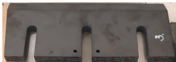
Fig. 2: Chopping knife coated with CROSAL + coating
