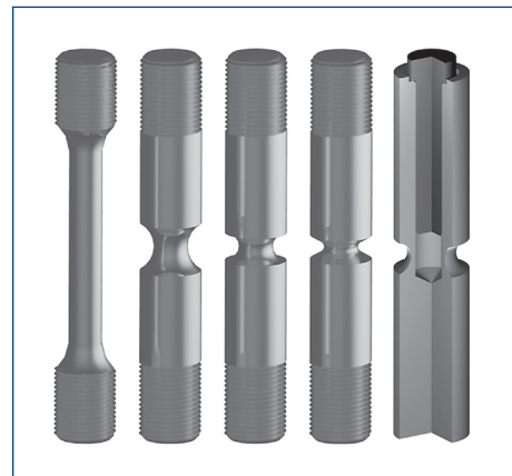
Figure 1. Geometries of cylindrical and notched tube specimens
