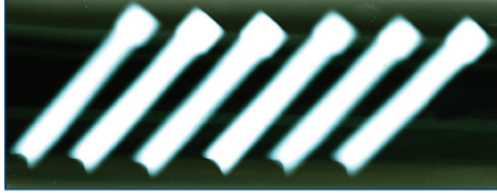
Figure 8. The X-ray of semi-products after the fifth reduction without chevron cracks
