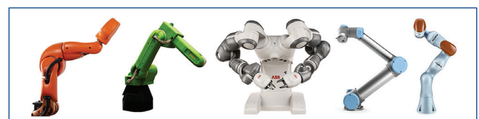
Figure 5. Collaborative robots – MRK-Systeme KR SI, Fanuc CR-35iA, ABB YuMi, UR5, KUKA LBR iiwa
