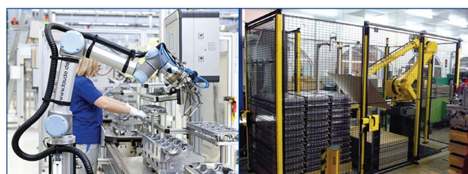
Figure 2. Robot workplace with collaborative (left figure) and conventional robot
