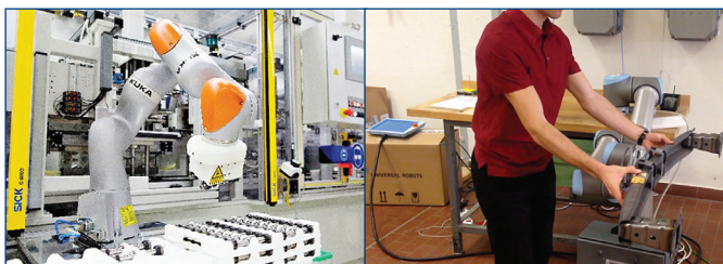
Figure 6. Collaborative robots in SKODA AUTO – KUKA LBR iiwa in Vrchlabi plant (left figure), testing of UR10
