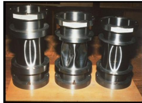
Figure 7. Shell instability of a circular cylinder
