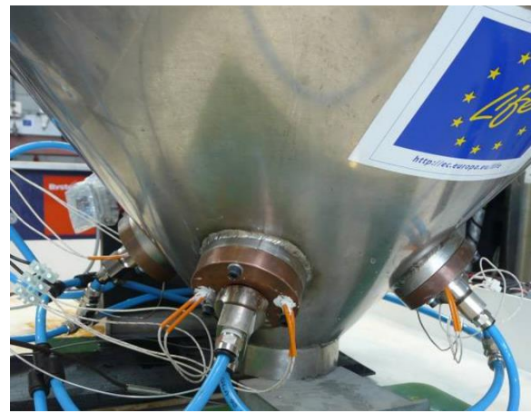
Figure 6. Vessel for ice particle generation with two copper heating rods and relays placed next to each water spray nozzle.
