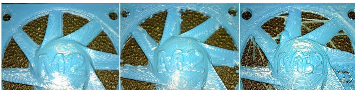
Figure 7. The real model made on the basis of data from the postprocessor (from Left) : Cura Engine, Slic3r, Skeinforge
