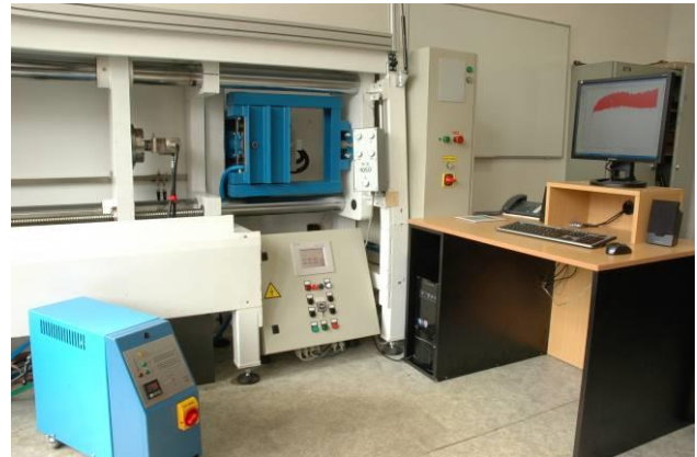
Figure 4. Equipment for tribological testing (SOKOL EVO II)
