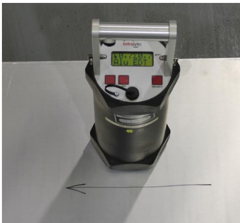
Figure 3. Measuring of lubricant amount by IR apparatus
