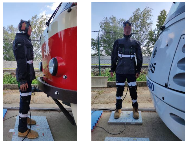
Figure 6. Examples of test setup (before disconnecting of the ATD data cable). T3 – front impact (left), 14T – lateral impact (right)
