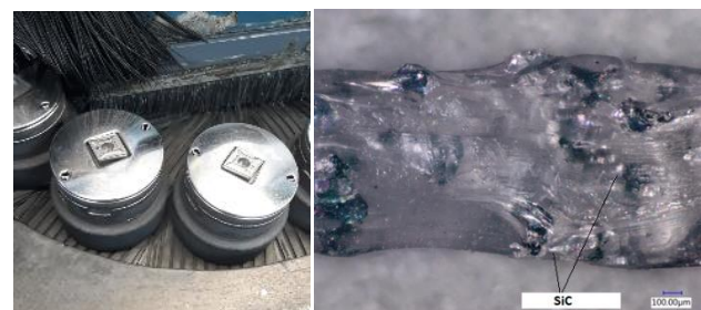
Figure 4. Inserts placed in a jig (on the left) and microscopic photo of brush tool 80SiC (on the right)
