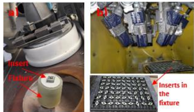
Figure 3. Dry blasting (a) and wet blasting (b) process
