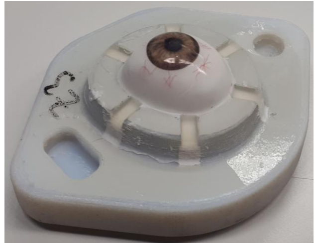
Figure 5. Silicone ocular prosthesis at the end of the production process within the casting mould
