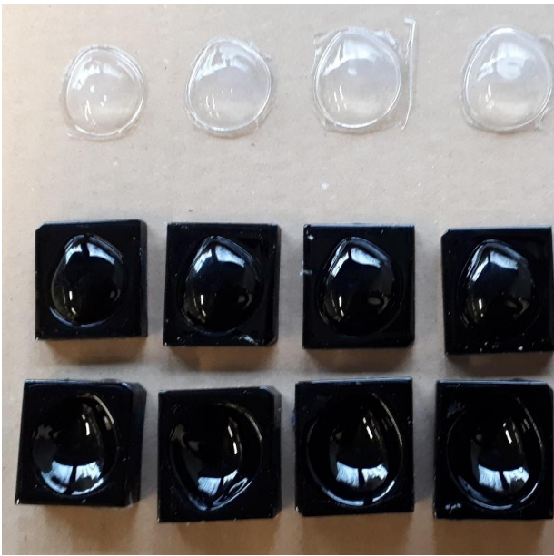
Figure 3. Shape cavities of prototype casting moulds
