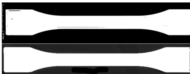
Figure 7. Section through the middle of linear manufacturing strategy (ECCS top, ZS bottom)
