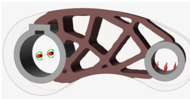
Figure 7: The new shape of the part with the application of the Shape Control function.
